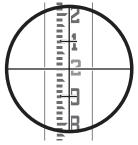
Distance measured in the figure:  $(1.347m - 1.042m) \times 100 = 30.5 m$ .
