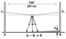
Set up the measuring tool in the centre and levelling rods **A** and **B** at both ends of the measuring distance. After aligning and focusing the measuring tool, read the heights at both levelling rods. Calculate the difference d between
