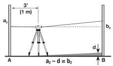
Set up the measuring tool approx. 6 ft (2 m) away from levelling rod **A**. After aligning and focussing the measuring tool, read the height  $\mathbf{a}_2$  at levelling rod **A**.
