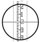
Height measured in the figure: 2.0 ft (1.195 m).
