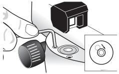
Check the circular bubble vial by rotating the telescope by 180°. If required, repeat the procedure or refer to an authorized SitePro after-sales service.
