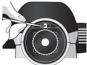
Unscrew the eyepiece cover **5**. Using the adjusting pin **18**, turn adjusting screw 5 clockwise or anticlockwise, until the calculated set value for height  $b_2$  is reached when measuring on levelling rod **B**.
